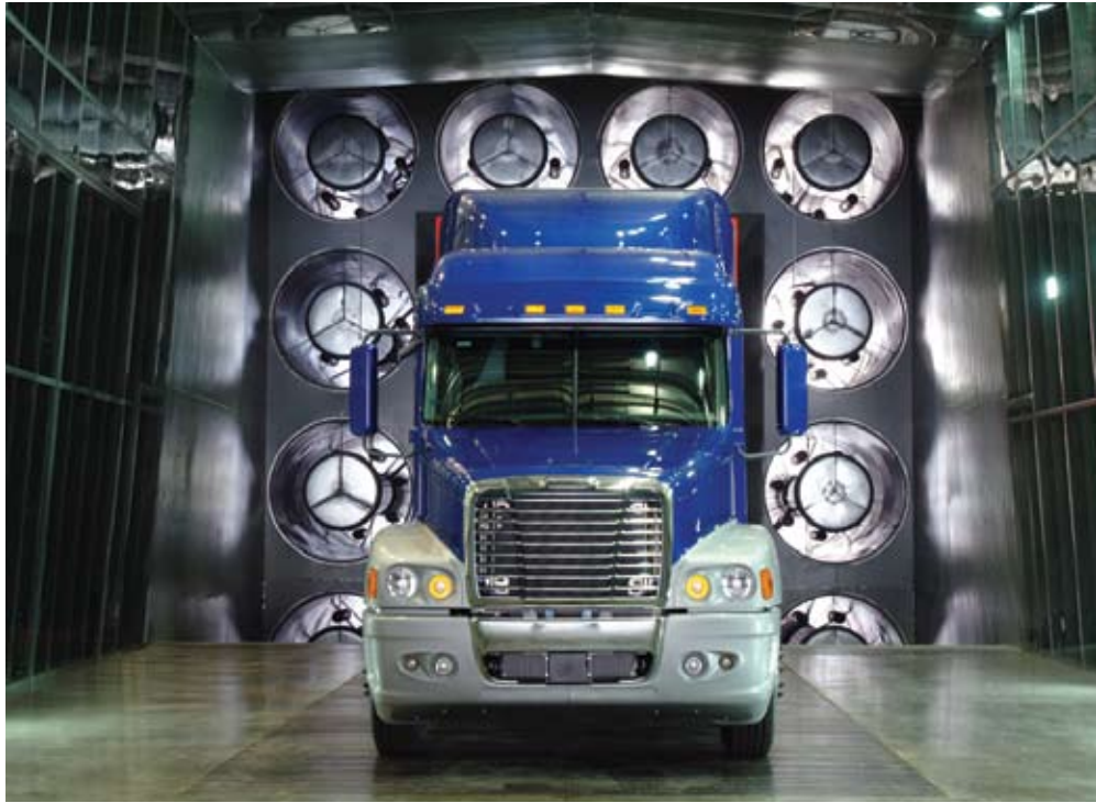
Freightliner LLC developed a Class 8 wind tunnel to conduct a two-year study on the impact of aerodynamics on fuel efficiency.
