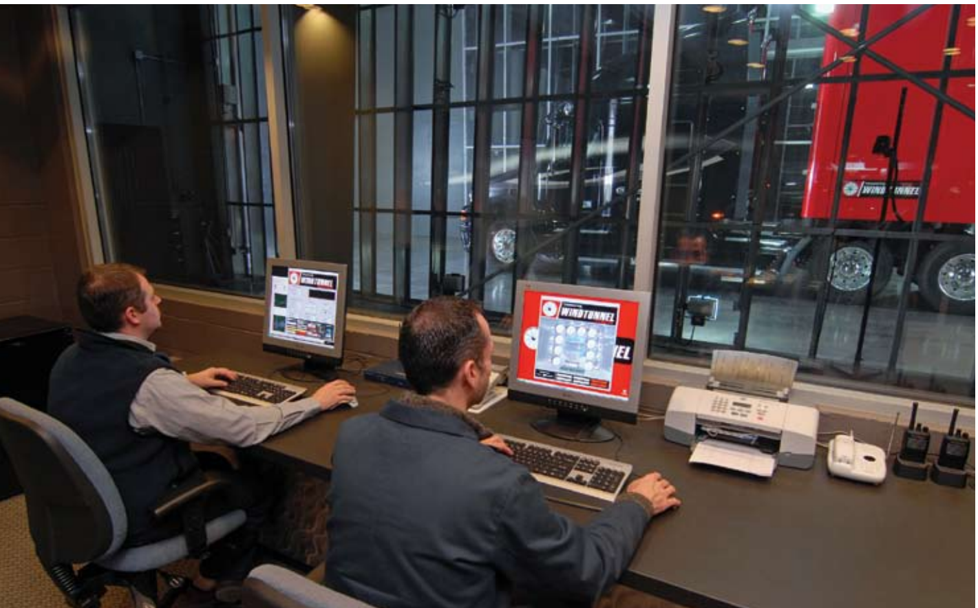
In the wind tunnel control room, Freightliner engineers are able to evaluate data collected in real time from both interior and exterior vehicle running tests.
